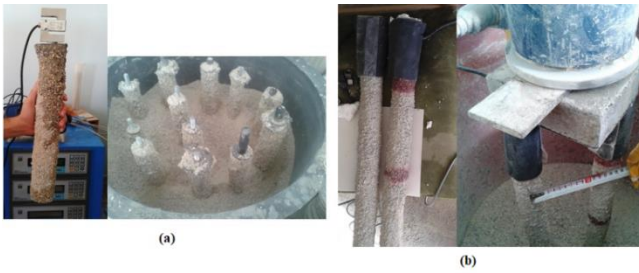
Figure 3 (a) D = 60 mm, L = 520 mm load cell placement on the pile and bolted pile production in different diameter, (b) D=50 mm, L=520 mm 150x150 mm installation of the piled raft (2 piled in the corner) into the tank [11]
