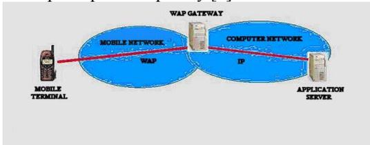
Figure 1. Working principle of WAP
