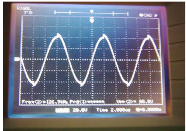
Fig. 8. 125KHz ( V_{pp}=98V ) sinusoidal signal obtained across the reader antenna
