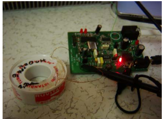
Fig. 7. The PCB photo of the reader circuit and antenna coil
