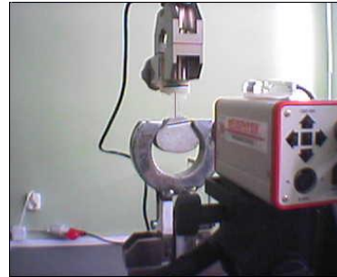
Figure 2.2.2 Pull-out experiment of single steel and glass fiber embedded into normal concrete.
