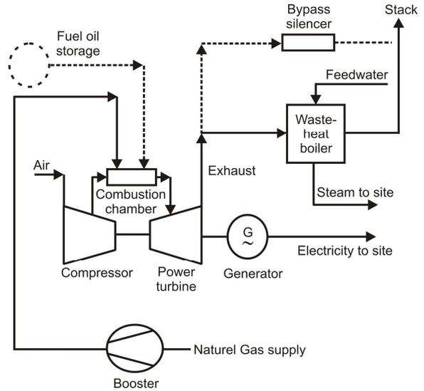
**Figure 4.** Block diagram of gas turbine based cogeneration power plants
