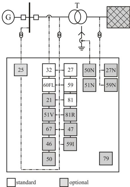
Figure 2. Typical multifunction interconnect relay
