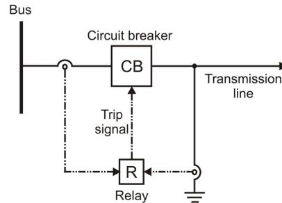
**Figure 1.** General protective relaying system
