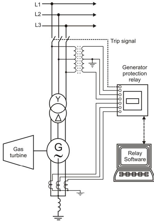
Figure 5. Reverse power data collection system
