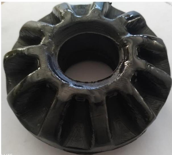
**Figure 10.** The forged bevel gear by using crank press (0.1 m/sec press speed).
