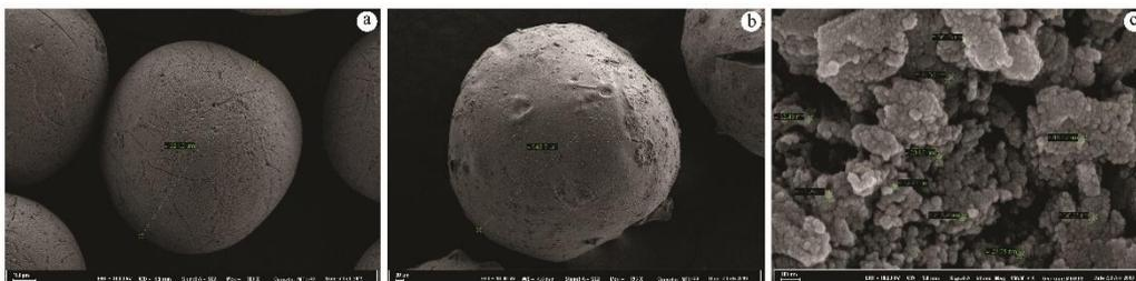
**Figure 2.** FE-SEM images of a) CS-GG microcapsules and b) Pd NPs@CS-GG
