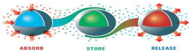
Figure 4 Phase change of PCM material in capsule during heat exchange [26].
