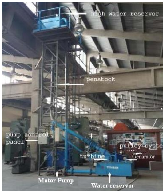
Figure 2. hydro-mechanical section general appearance.
