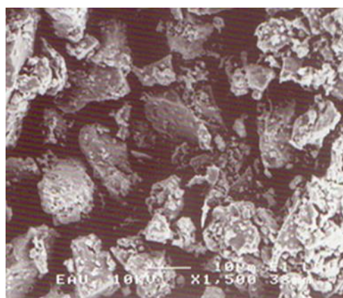
Figure 2. SEM photogram of the chalcopyrite concentrate.
