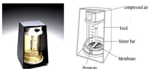
Figure 1. UF cell used in the experiments.
