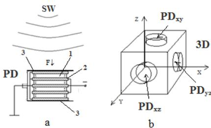
**Fig. 3.** Design of a single-dimensional PD (a) and 3D-dimensional (b) piezoelectric detectors: 1–piezoelectric plates; 2–foil layers, 3– insulating layers; PD<sub>xy</sub>, PD<sub>xz</sub> and PD<sub>yz</sub> are piezoelements allocated on the XY, XZ, and YZ planes, correspondingly; SW- seismic wave.
