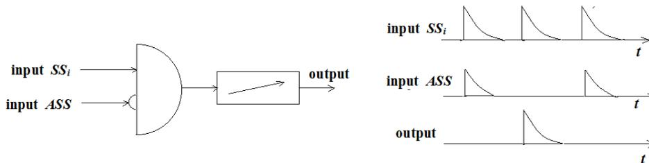
**Fig. 7.** Anticoincidence circuit.
