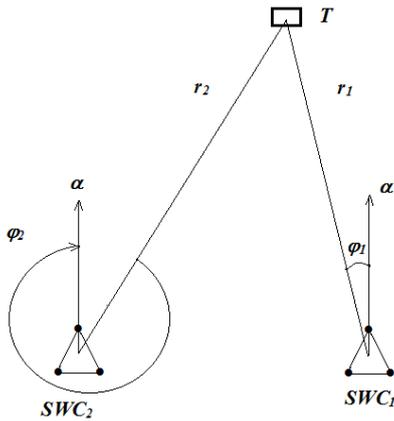
**Fig. 5.** The determination of the target location by triangulation:  $r_1$  and  $r_2$  are distances to target  $T$ ;  $\alpha$  is a reference direction;  $\varphi_1$  and  $\varphi_2$  are directional angles.
