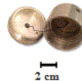
Fig. 1. Piezoelectric detector.
