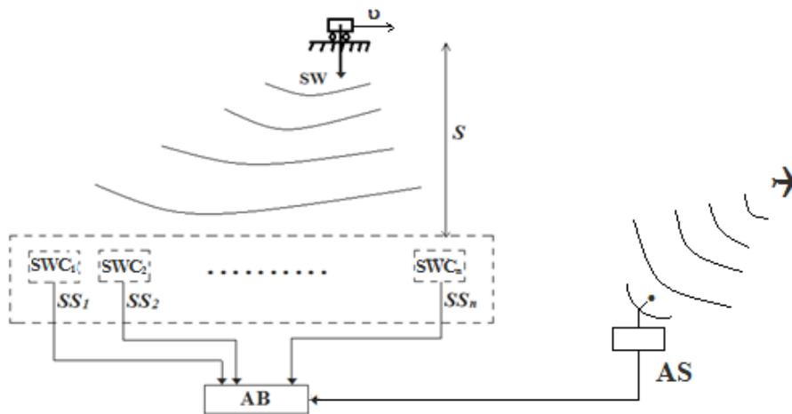
**Fig. 6.** Seismic location station SLS. SWC<sub>1</sub> - seismic waves cells; SS<sub>i</sub> – output signals from SW<sub>i</sub>; SW – seismic waves from moving truck;  $v$  - velocity of truck; S – distance to moving truck-target; AB - analyzing block; AS-acoustic system.
