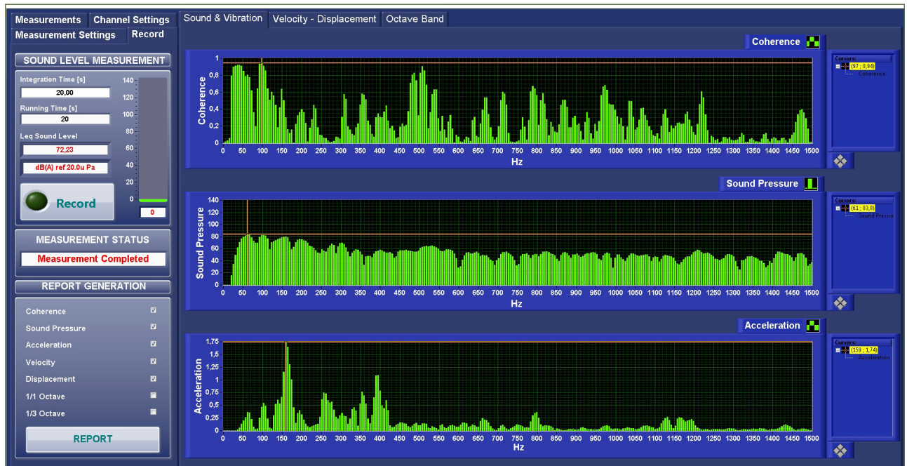
Figure 3. A screenshot of the user interface of the developed test software
