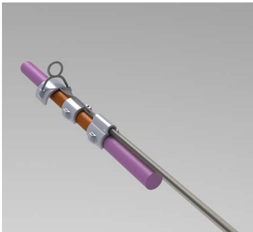
Figure 2A: Implanted bipolar electrode. user friendly cuff contacts (not wrapped around the nerve)
