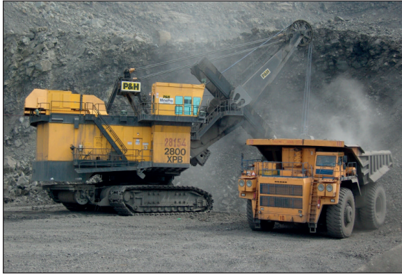
Photograph 2. Dig segment of cycle time of a 35 m 3 electric rope shovel (Anon (b), 2015)
