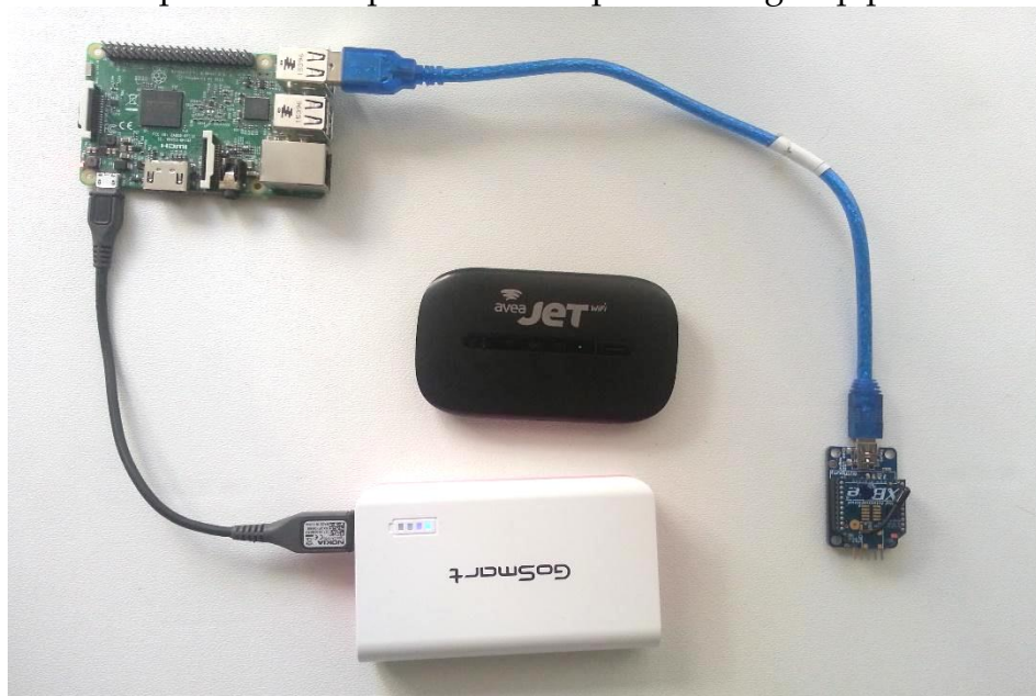
Figure 1: Central Control Unit using Raspberry Pi-3
