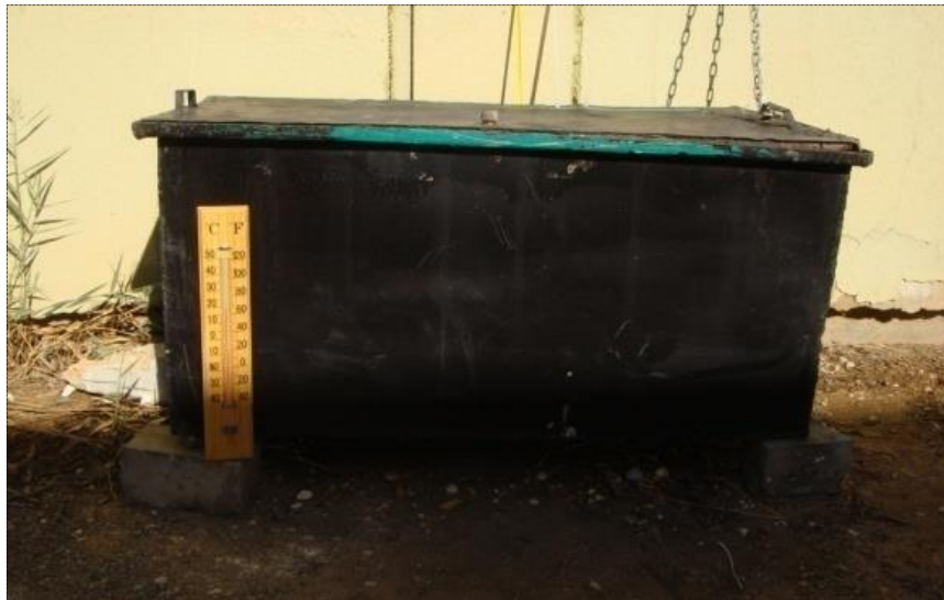
Figure 2. Steam Curing Chamber
