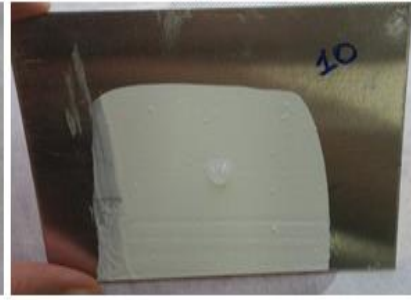
Figure 12. Flow appearance of sample with aerogel as a paint additive for water based paint
