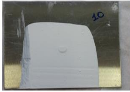
Figure 11. Sample with aerogel as a paint additive for water based paint
