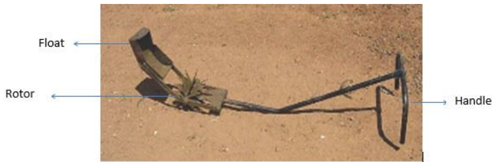
Figure 1. Pictorial view of Mandava single row weeder (Ravi, 2000)
