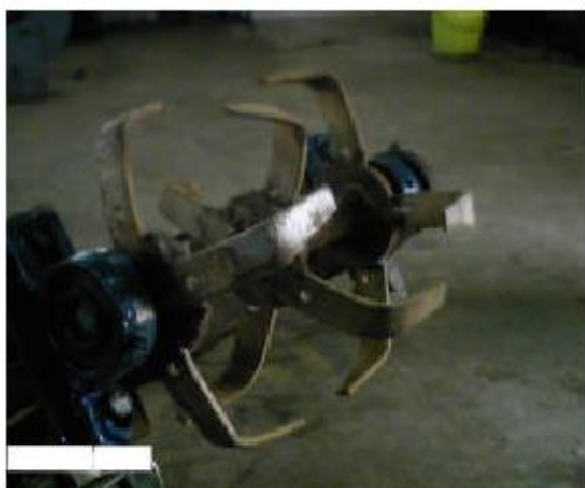
Figure 9. Cutting blade of the row crop mechanical weeder (Manuwa et al., 2009)
