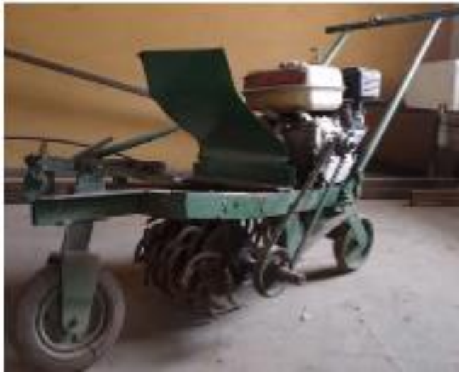
Figure 13. Isometric view of a power rotary tiller (pictorial view) (Olaoye and Adekanye, 2011).
