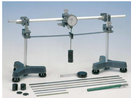
Figure 1. Beam deflection apparatus (Pisačić et al., 2018)
