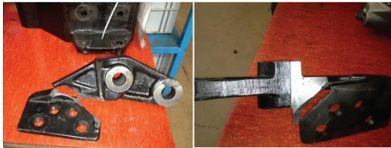
Figure 13- Brackets breakage points at the push-pull tests
