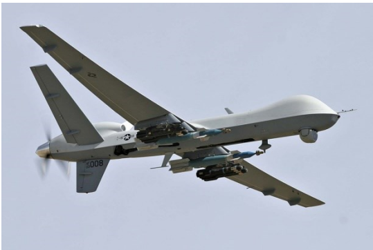
Fig. 1. Predator B turboprop UAV [1].
