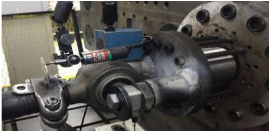
Figure 5. Test Setup for Radial Stiffness
