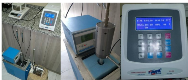
Figure 2. Preparation of nanofluid with temperature control
