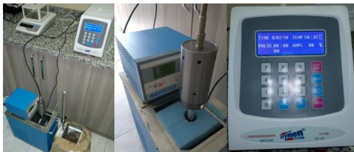
Figure 2. Preparation of nanofluid with temperature control
