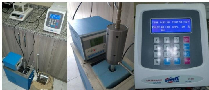
Figure 2. Preparation of nanofluid with temperature control
