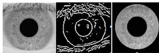
Figure 5. Determining circular borders and noise [13, 41]
