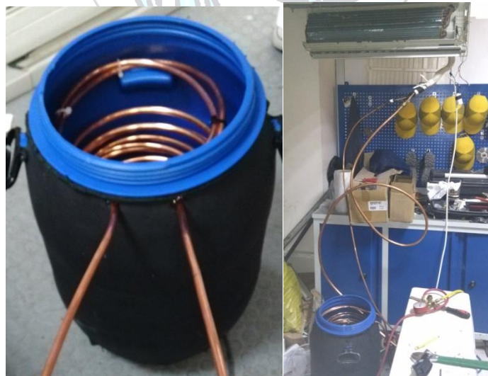
Figure 2. Designed boiler unit and assembled experimental setup
