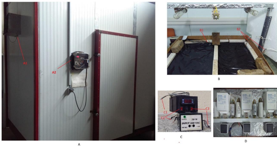
Figure 2- Representation of the equipment used in conducting experiments to record the changes in soil temperature and humidity. A: Temperature isolation chamber (A1: Air conditioning fan A2: Electronic board setting of temperature and startup of heating and freezing system). B: The space above the soil bed (B1: The location of the connection cables to the sensors B2: The entrance of refrigerant pipes to a depth of 40 cm). C: The system for installing a heating and freezing system at a depth of 40 cm (C1: PT100 temperature sensor, C2: key and connection to the coolant flow regulator pump, C3: key and connection to the thermal plate embedded at a depth of 40 cm). D: Electric circuit for HPS bulb startup: Capacitor, ballast and Igniter for each bulb
