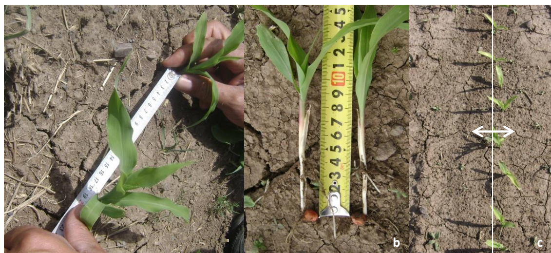
Figure 2- Measurements of intra-row spacing (a), sowing depth (b) and deviation from the row (c)
