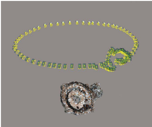
Figure 2. Camera stations configuration of turbohousing (inside)
