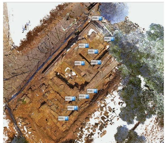
Figure 5. Alignment workflow of the point clouds; data from TLS.
