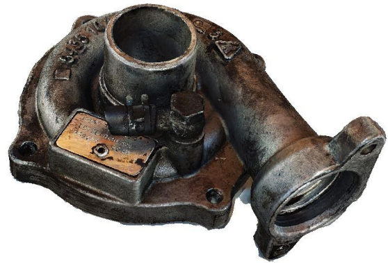
Figure 9. Turbo-housing dense point cloud obtained by ContextCapture
