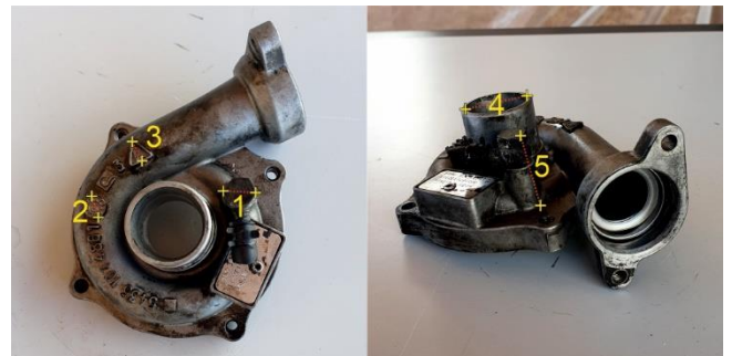
Figure 17. Detail measurements for accuracy assessment (Compressor housing)
