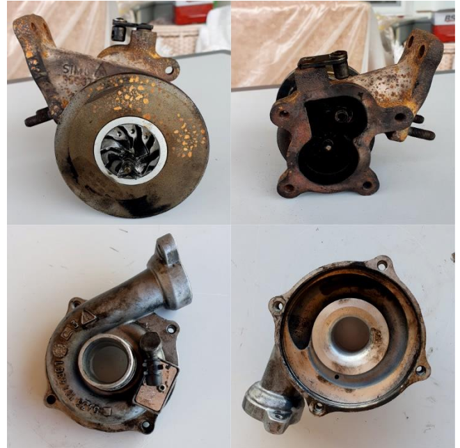
Figure 1. Damaged turbocharger of 2004 Ford Fusion TDCi – separated into components
