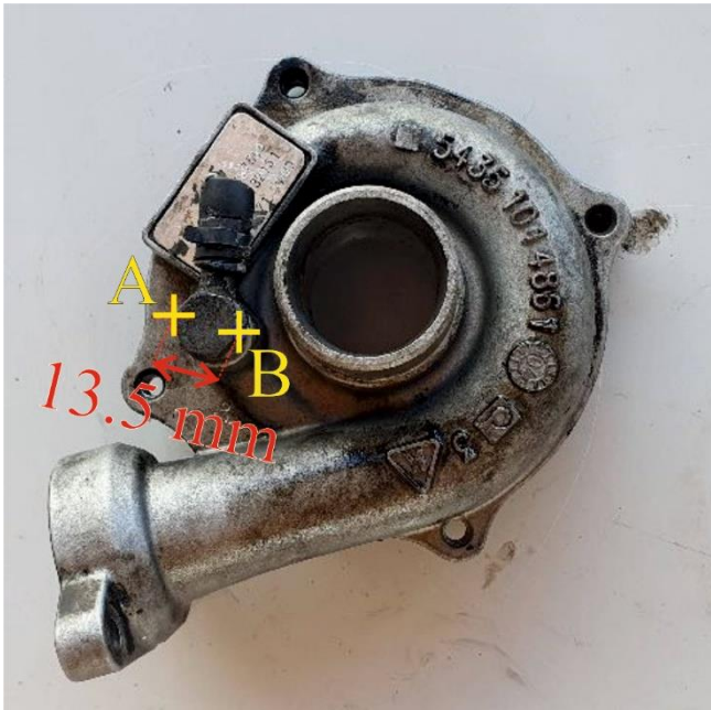
Figure 8. User tie points and scale constrains of the turbo-housing (outside)
