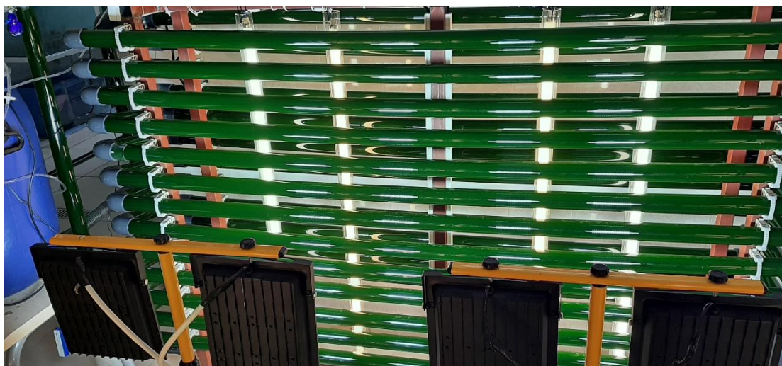
Figure 1. Chlorella sp. production at tubular PBR
