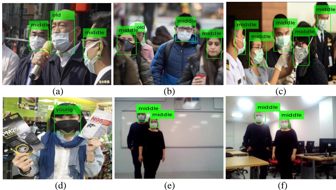
Figure 6 Some samples of the system output from Face Mask Dataset (a,b,c,d) and real time test environment (e,f)
