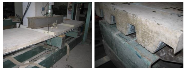
Figure 9 Testing of single span bending tests
