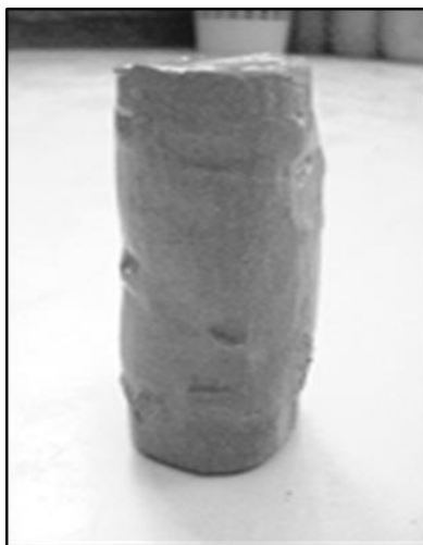
b) Typical sample after testing in Triaxial
