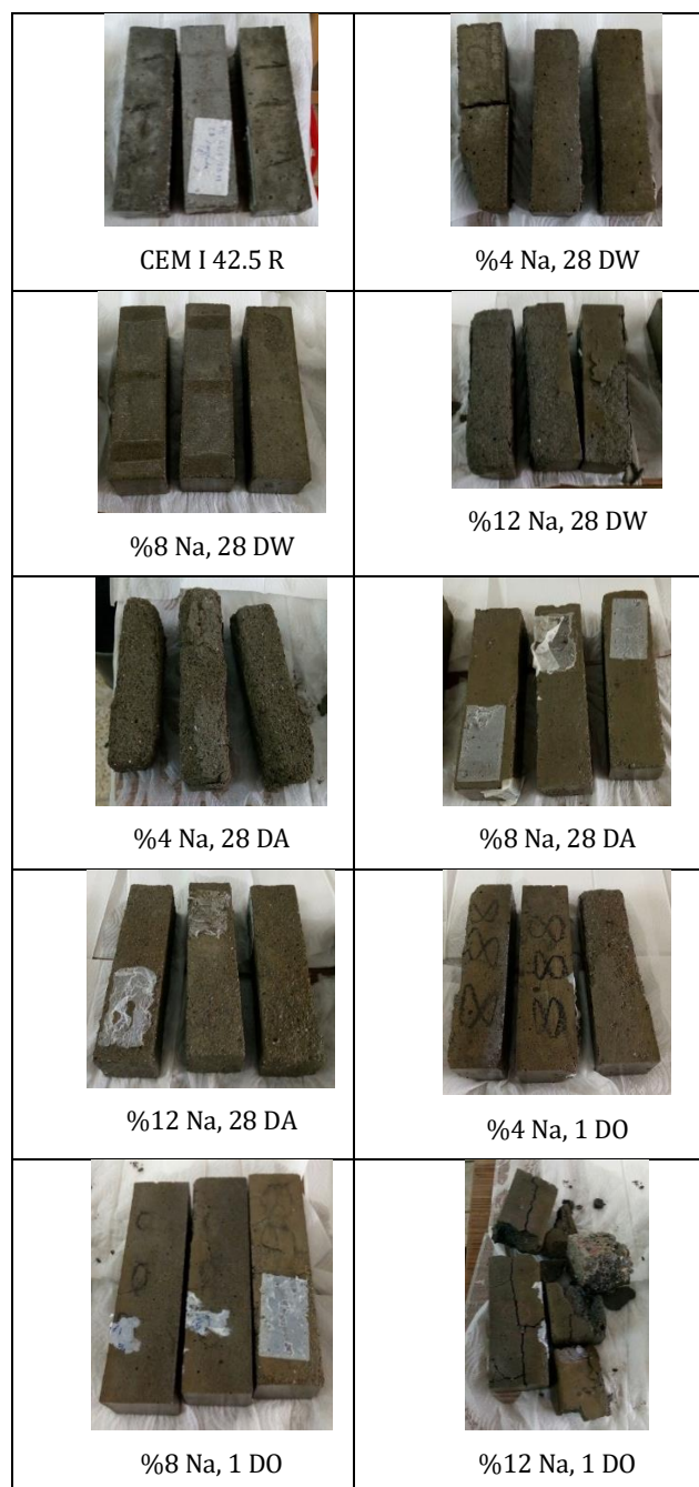
Figure 1. Images of mortars after freeze-thaw test
