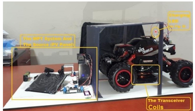
Figure 11. Prototype imaging of the designed wireless charging station
