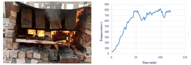
a). Damage by fire b). Temperature and time
