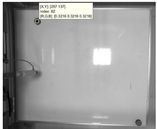
Figure 9. Pixel values corresponding to the point (0,0) used on the machine are shown
