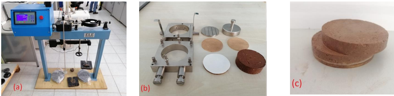
Figure 5. (a) Shear box assembly. (b) Compacted specimen, porous stones and cutting box apparatus. (c) Visual of the sample after the test
