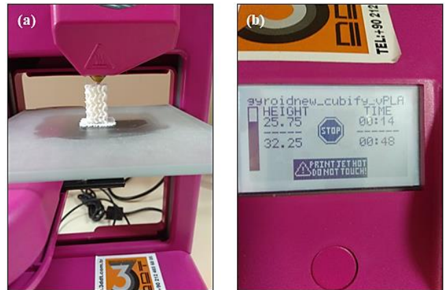
Figure 4. Pictures of (a) the 3d printing process of the PLA scaffold and (b) the screen view of the 3d printer during the printing procedure
