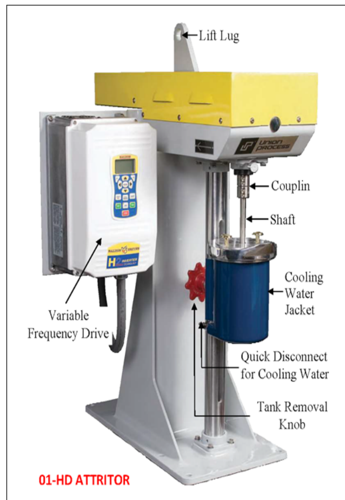
Figure 1. The Model HD-01 stirred ball mill used in the experiments
