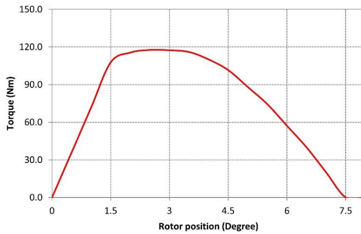
Figure 7. The graph of the torque generated by a phase at the nominal current depending on the rotor position.
