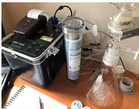
Figure 1. Zeolite Filter Radon Test Device RAD7.
