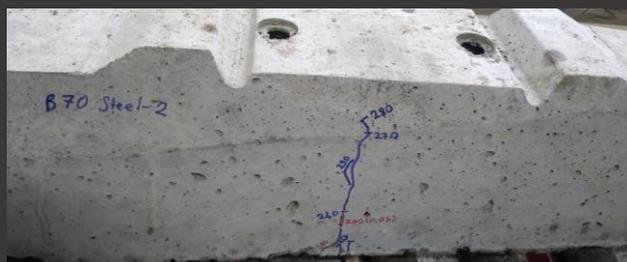
Figure 9. Cracks occurred at the first crack formation load (Fr = 210 kN) and permanent crack load (Fr0.05=290 kN) after the test load is removed
