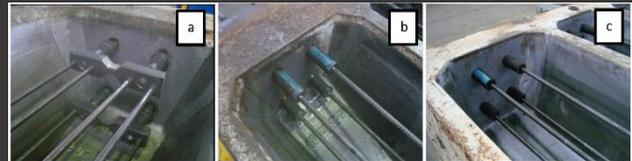
Figure 3. Various reinforcement and anchorage mechanisms in carousel sleeper production system a. Without ribbed-with anchor plate, b. Ribbed-with anchor plate, c. Ribbed-without anchor plate [3]
