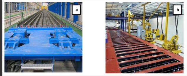
Figure 2. Common production methods of pre-stressed reinforced concrete sleepers: a. Pre-stressed sleeper production with long-line system b. Pre-stressed sleeper production with a carousel system
