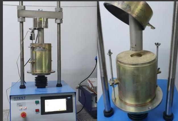
Figure 3. Automatic CBR test machine
