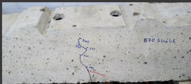
Figure 8. First crack formation (Frr = 190 kN) and permanent crack load (Fr0.05=300 kN) after the test load is removed
