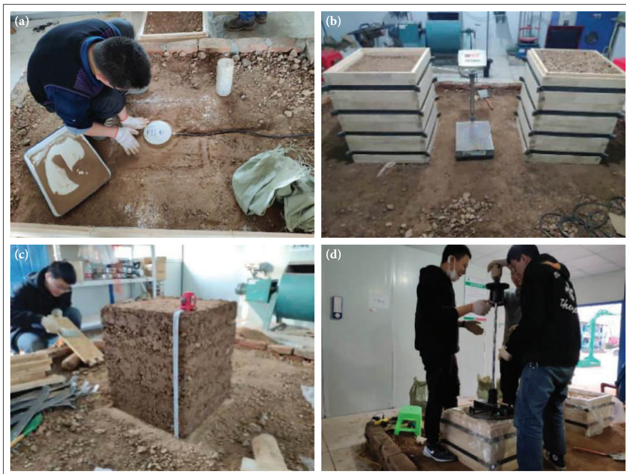
Figure 5. Dynamic, resilient test for compacted CGS fillers in laboratory. (a) Installation of earth pressure cell. (b) Parallel tests with molds. (c) Stacked models without mold. (d) Dynamic impact loading.
