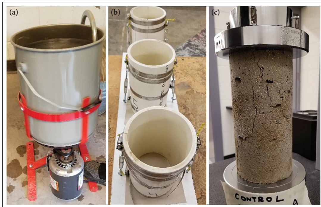
Figure 3. (a) CLSM mixer; (b) Specimen mold; and (c) Unconfined compressive strength test setups.
