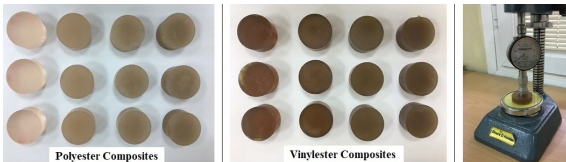
Figure 3: Shore D hardness testing of polyester and vinylester composites.
