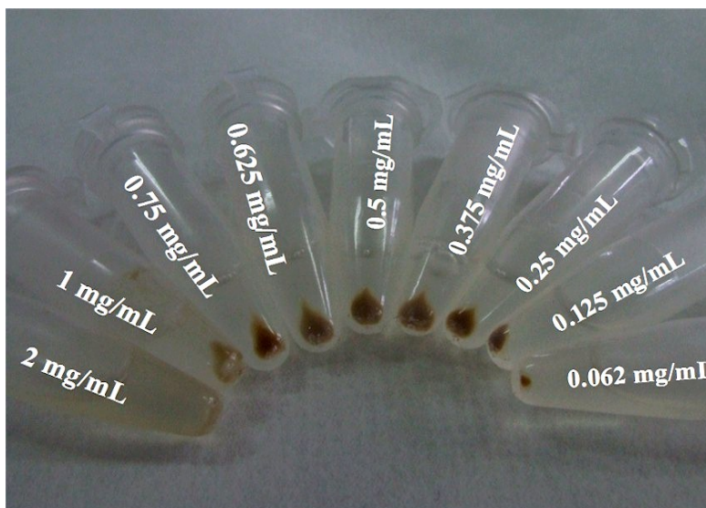
Figure 2: Degrees of PEI-lipase precipitates obtained at varying PEI concentrations (different PEI to lipase mass ratio) after centrifugation at 10,000 rpm for 2 min.
