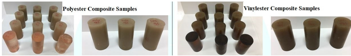
Figure 2: Tincal-reinforced composite samples before and after compressive strength test.
