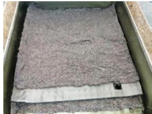
Figure 6 The third geotextile felt moisture trap placed on the root retaining layer
