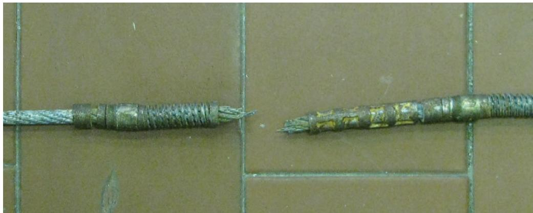
**Figure 12** - Diamond wire breakage at the iron joint.
