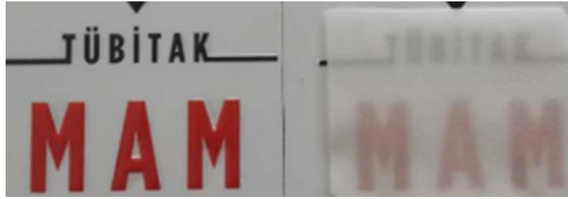
Figure 6. Five layer tapes sintered at 1650 °C.
