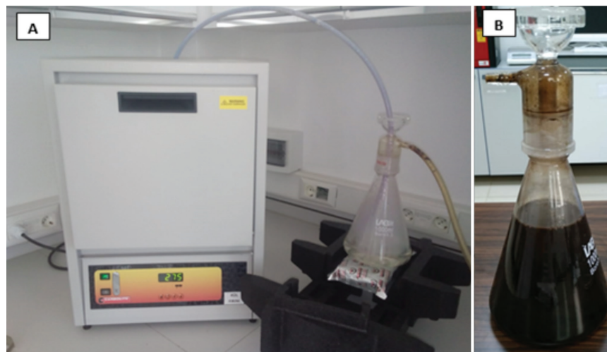
Figure 4- A) The process of burning the Medicago sativa L. straw in the laboratory oven, B) The smoke water obtained
