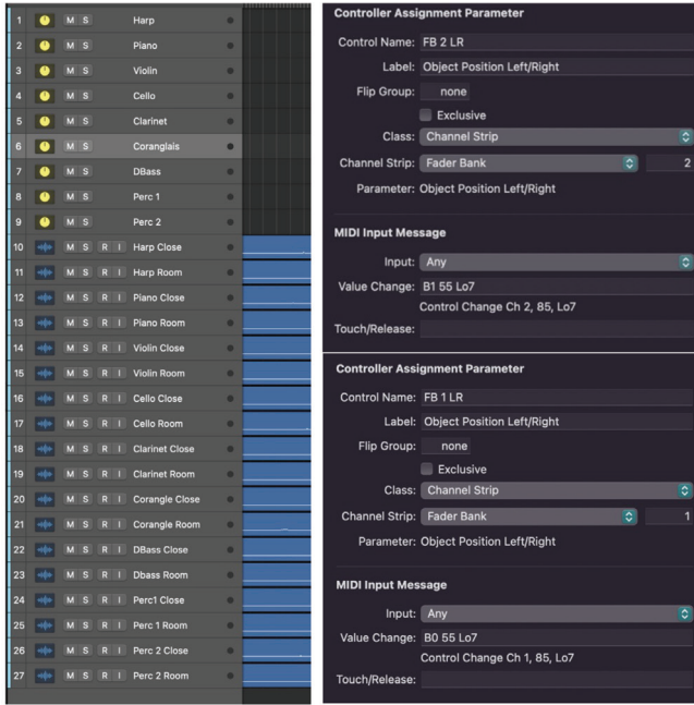
Figure 13. a) Channel order in Logic Pro (left) b) MIDI mapping in Logic Pro (right)
