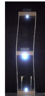
(a) (b) (c) Figure 18 First mode shapes. a) Video frame with maximum displacements, b) first mode shape obtained experimentally, c) first mode shape obtained theoretically.
