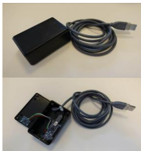
Figure 2 Outside (left) and inside (right) views of the low-cost Arduino-based accelerometers
