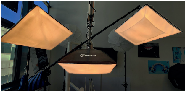
Figure 1: Recommended setup no 1 including 3 paraflashes at fixed positions above the dental unit.
