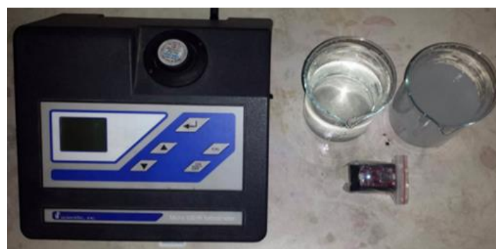
Figure 4. The turbidity meter, two water cans containing pure water and turbid water respectively, and the redbear due board.
