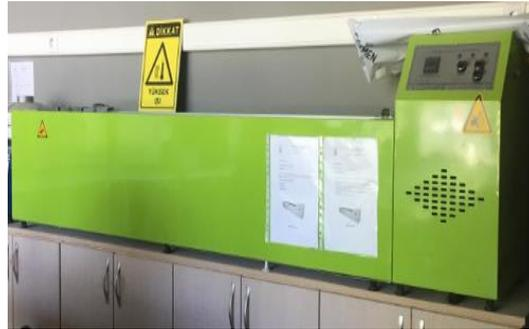
Figure 10. Ductility Test Device
