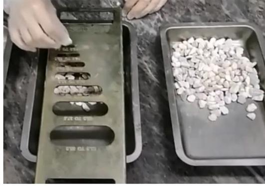
**Figure 3.** Flatness Index Determination
