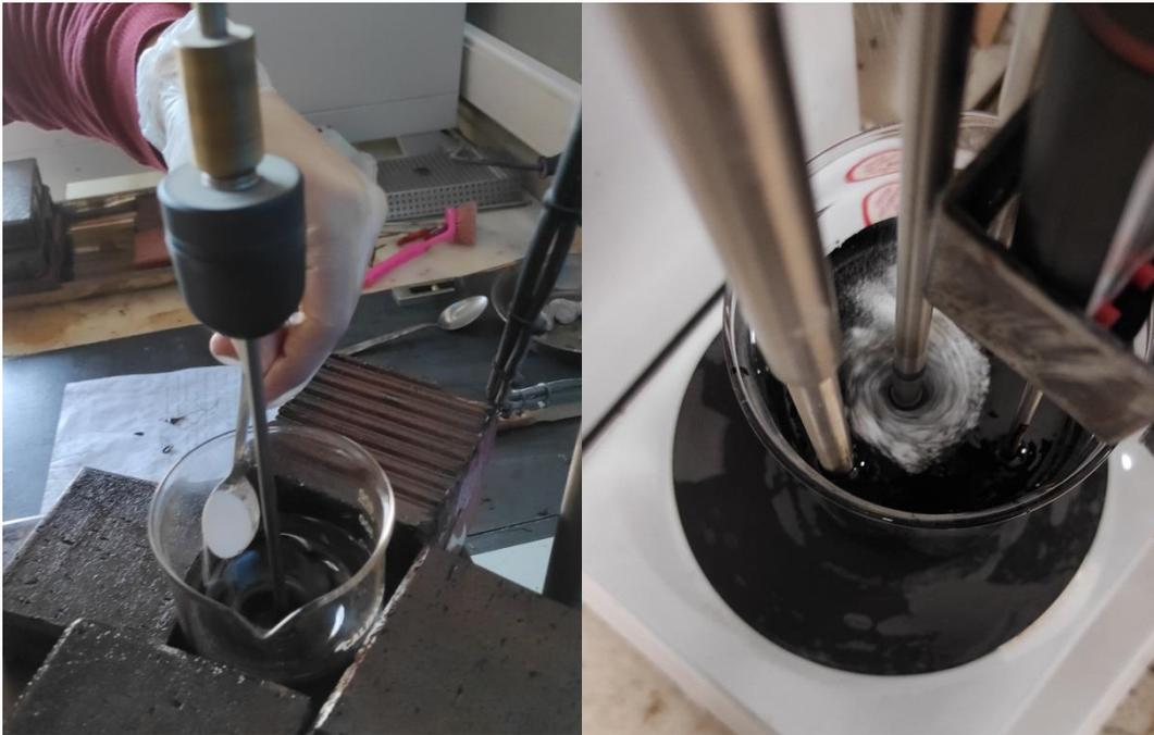
**Figure 6.** Production of PVC Waste-Modified Bituminous Material
