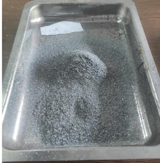
**Figure 5.** PVC waste additive
