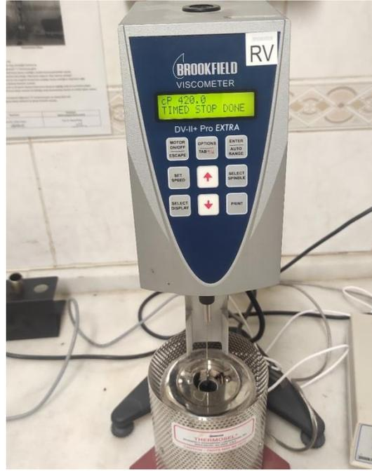
**Figure 14.** Brookfield Viscosity Test Device
