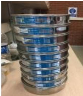
**Figure 1.** Set used in sieve analysis
