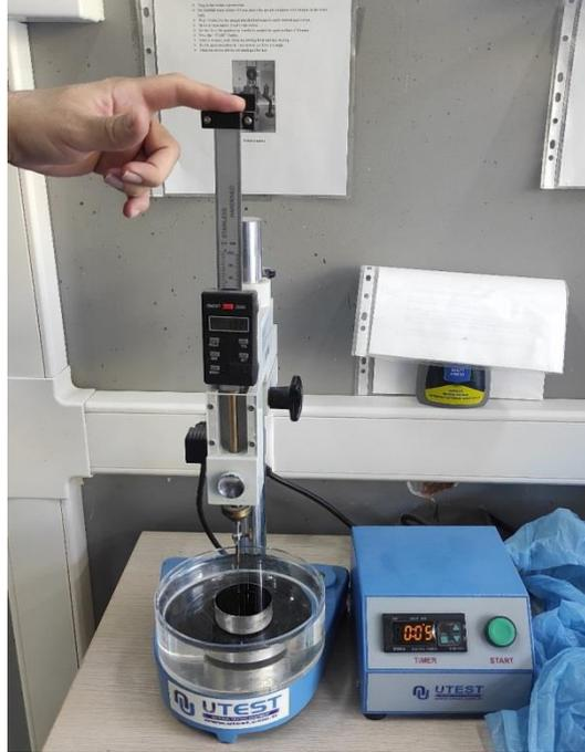
**Figure 7.** Penetration test machine
