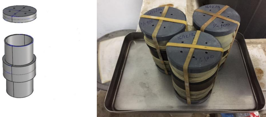
Figure 2. Modified steel mold 3-D view and prepared sample in the modified steel mold.
