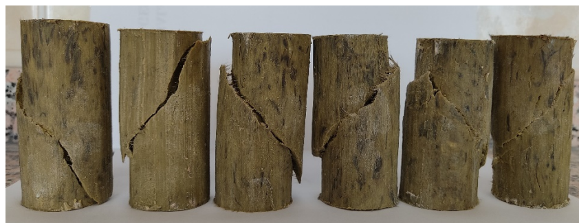
Figure 7. Samples after unconfined compressive test.
