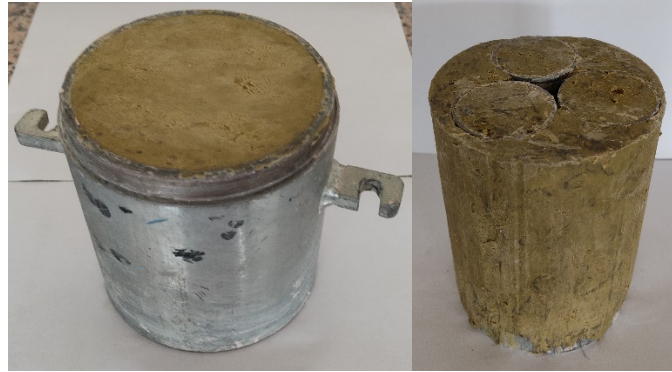
Figure 4. Proctor test and taking cylindrical samples.
