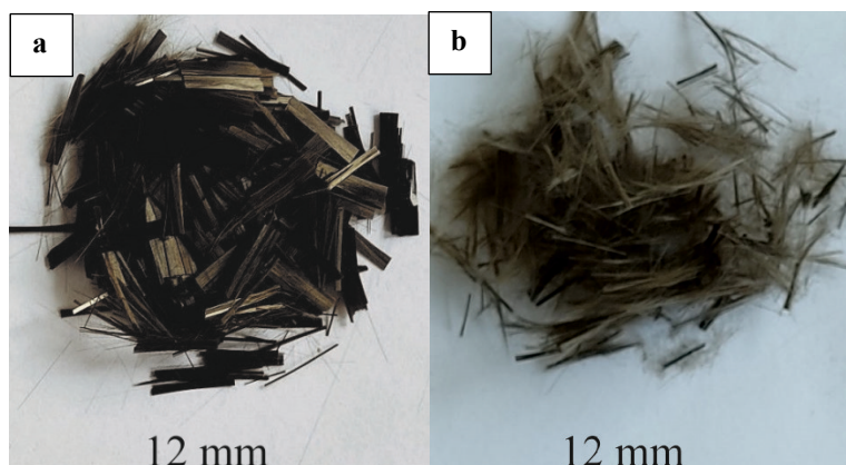
Figure 2. Unseparated (a) and separated (b) basalt fiber used in the study.
