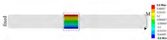
Figure 4. Bending stress of cantilever beam (in MPa).
