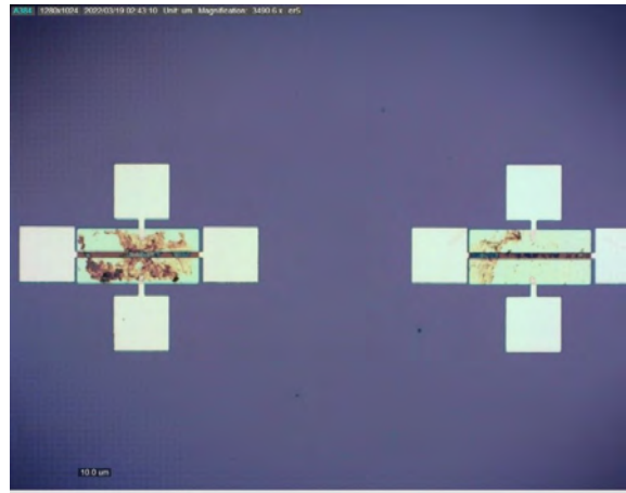
Figure 9. Top view optical microscope photograph of micro memristive device after graphene patterning with optimized lift-off
