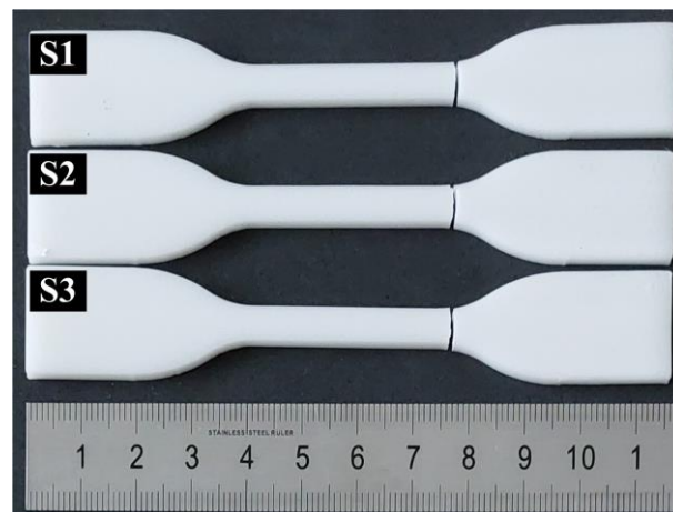
Figure 5. Specimens after the tensile test
