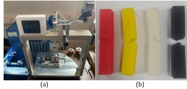
Figure 3. a) Charpy impact test device in the study and b) samples
